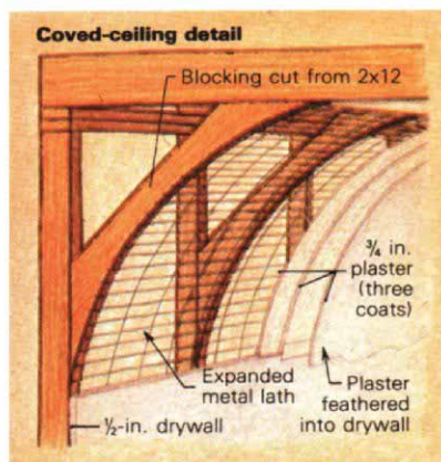
An inside corner of the coved ceiling. Curved ribs were cut from 2x12s, as at left. These ribs were covered with expanded metal lath, the base for three coats of plaster.
